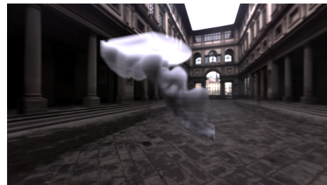
Figure 10: Result of a 128^3 participating medium lit by an environmental map. It took 2291 ms to compute 3 scattering orders with 25 propagation directions.
