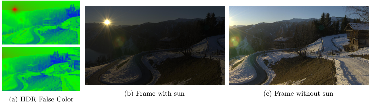
Figure 1: Illustration of lack of temporal coherency in video tone mapping. On the false color representation (a), red represents the maximum HDR value of the video while blue its minimum. Both frames have the same HDR values between similar regions. However the scene (c) appears a lot brighter than the scene (b). Furthermore, the perception of the landscape is different between the two frames.
