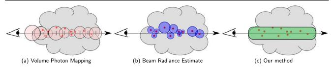
Fig. 1 Different ways to gather photons. Regular ray marching (a) may take into account several time a same photon whereas *Beam Radiance Estimate* (b) and our method (c) gathers all photons once and for all
