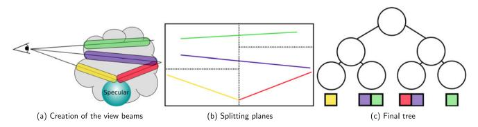
Fig. 3 Example of a view beam Kd tree building for a set of beams (a). Only the supporting rays are used in the tree (b). Some leaves (c) contains several beams, and beams crossing splitting planes are duplicated in the tree
