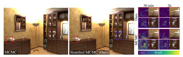
**Figure 1:** Our stratified MCMC shows less noise than primary sample space MLT (PSSMLT) [KSAC02] in the same rendering time (30 minutes). PSSMLT gets stuck exploring only a portion of the image while our technique produces more predictable results. This translates to a lower mean absolute percentage error (MAPE) across the whole image.
